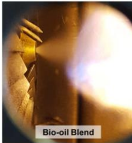
Figure 1. Burner flame on bio-oil (left) and diesel fuel (right)
