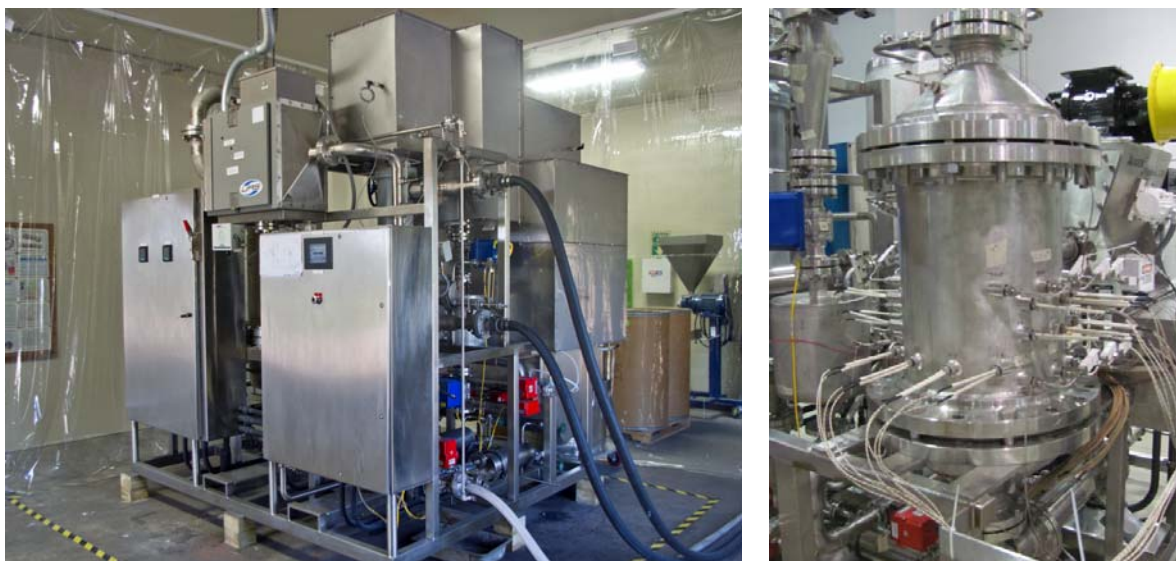
Figure 3. Pilot-scale fast-pyrolysis reactor (45 kg/hr)
