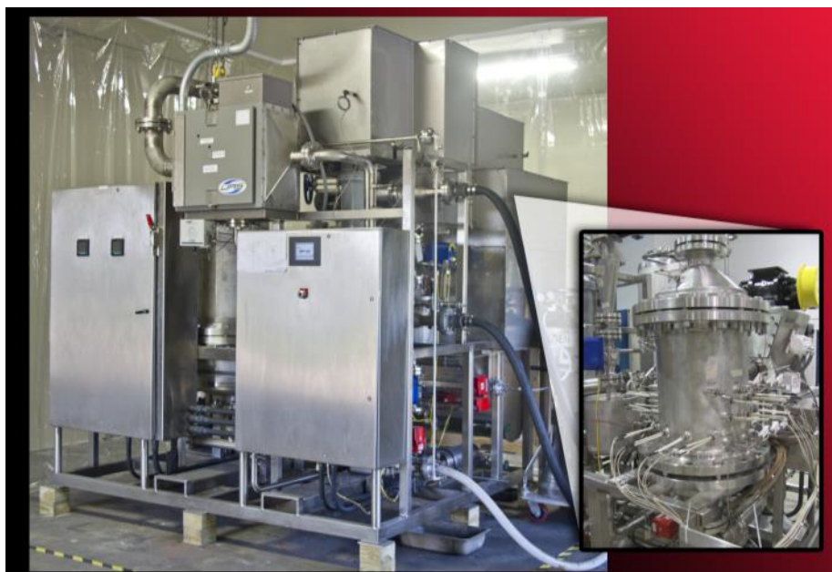
Figure 2: Pilot-scale fast pyrolysis process during laboratory testing (bubbling fluidised bed reactor shown in inset).
